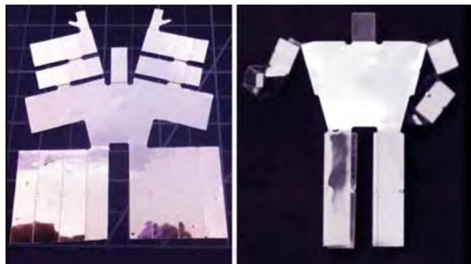
*The bakeable robot as its name infers, assembles itself when extreme heat is applied to it; the basic structure is pre-printed and mapped out so that when it is heated, it folds into its three-dimensional form*
