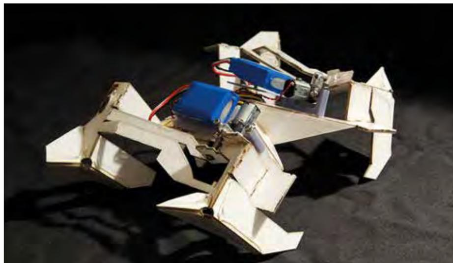
*The self-folding mobile prototype developed by researchers at MIT and Harvard: These robots have potential for both medical applications and in crisis response, especially where the usual protocols and procedures are limited by the surrounding environment and circumstances*
