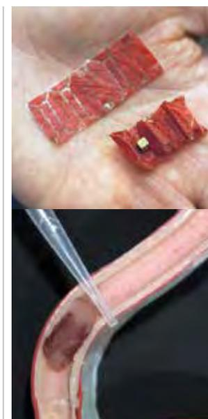
*The ingestible robot is swallowed via a biodegradable capsule (made of ice or other organic material) and is activated via biological interaction with stomach fluid. The folding process is initiated by gastric liquid after which the robot can then be steered by external magnetic fields*
