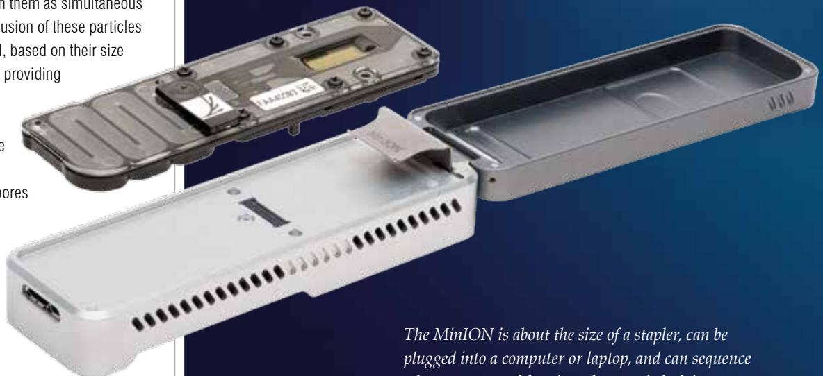
*The MinION is about the size of a stapler, can be plugged into a computer or laptop, and can sequence a large amount of data in a short period of time*
